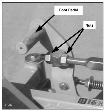
Deck Level Adjustment Foot Pedal Figure 3-19
